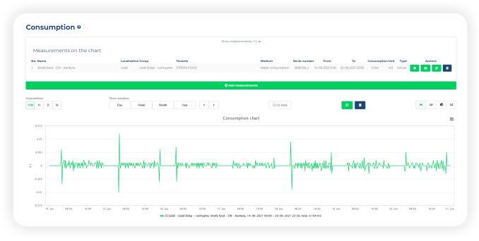
Additionally, in the case of the Food zone meter WM-05 CW FOOD, what matters is the pulse value (the pulse weight) of the virtual meter. If the impulsing of the master meter is different than that of the subordinate meters, than a short interval (15-minute) chart may show distorted data.
